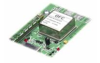
The Ovenized Crystal Oscillator (OCXO) upgrade improves holdover accuracy. By keeping the crystal oscillator at a fixed temperature, if the GPS signal is lost, thereby placing the server in holdover, the OCXO reduces clock the drift.
