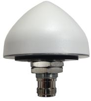
The antenna used with the SyncServer S600/S650 is a high-gain (40dB) GNSS antenna covering the GPS L1, GLONASS L1, and SBAS (WAAS, EGNOS and MSAS) frequency band (1575 to 1606 MHz). The antenna has a three stage low-noise amplifier, with a mid-section SAW with a tight pre-filter to protect against saturation by high level sub-harmonics and L-Band signals making it excellent for timing applications. An L-bracket for pole mounting and 3-foot BNC(m) to N(f) cable is also included.
