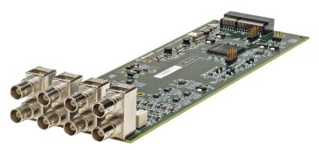
The Timing I/O Module is an exceedingly versatile time and frequency input and output option. In the standard configuration, it supports the most popular input and output time codes, sine waves, and rates. In the table below, the user can see the standard configuration, and the configuration with the FlexPort™ option.
